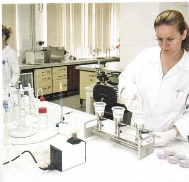
Membrane Fiter filtration system in operation
